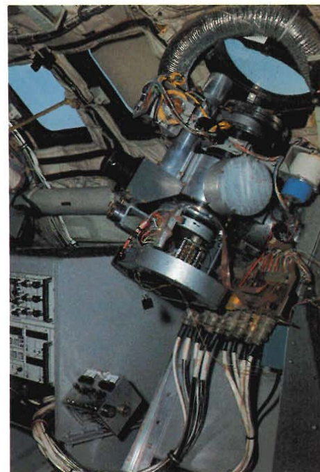
Fig. 10. Los Alamos-designed telescope for photographic polarimetry and electronic control equipment (lower left) mounted in aircraft. This instrument photographs the corona beyond 12 R_{\odot} and has provided data for determining electron densities and image-enhanced photographs of the outer corona. (See note "Unique Record of the Changing Corona.") The blue cylinder (upper right) is one of three orthogonally mounted gyroscopes obtained from NASA's Apollo program. These provide the inertial references that allow this instrument to point at high accuracy even when the aircraft is in motion.
